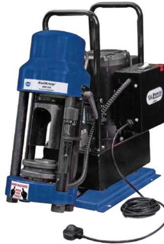
KuriCrimp™ KD165 Has a 60 ton press, crimps 2 and 4 wire hose up to 1 1/4" and 6 wire up to 1" ID. 2 wire braided and ABT4K up to 1 1/4" and ABT5K up to 1" ID.
