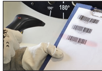
Barcode Reader instantly calls up saved crimp diameter
