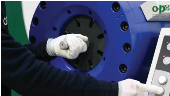
Master dies are guided through built-in channels on the tool on mid-sized crimpers.
