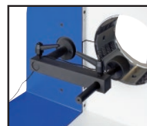
Back Limit Switch
